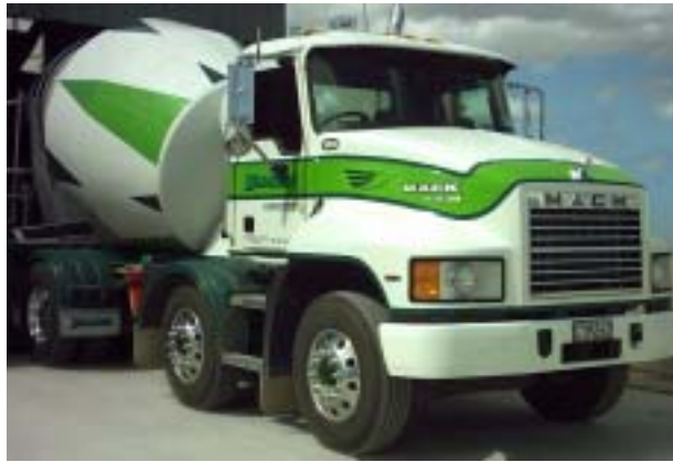
Higgins recently added 4 of these large concrete trucks to add to their fleet of 35. They each hold 6.4 cubic metres of concrete compared to normal truck loads of about 5 cubic metres.
